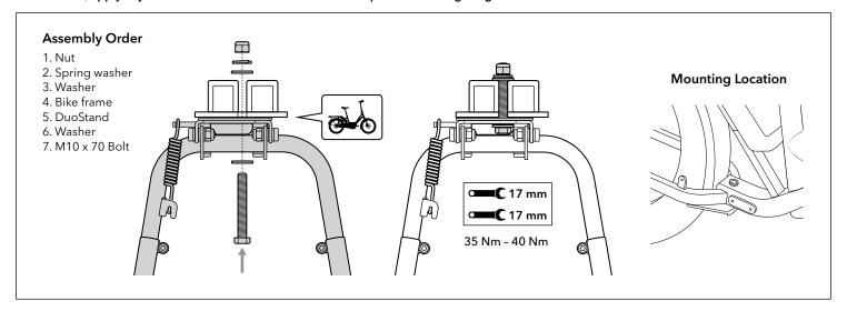
3. The recommended clearance from the bottom of the rear wheel to the ground is 10 - 15 mm (3/8" - 5/8"). Measure the distance from the bottom of the rear tire to the ground and adjust the height of the DuoStand by loosening the bolts on the DuoStand Ends to raise or lower the legs. Tighten the bolts to a torque of 8 - 9 Nm.
